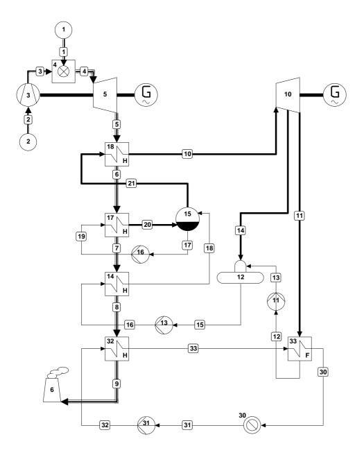
Figure 4-1: STAG-unit with back-pressure steam turbine
